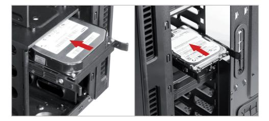
Please note that 3.5 inch disk are inserted into the cage from the left side as seen from the front and the 2.5 inch drives from the right side as seen from the front.
