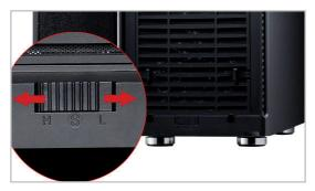
The Cooltek Antiphon offers a **two**way fan controller for up to three fans at the lower end of the front. You can choose between **High** speed for maximum case ventilation or Low speed for silent operation of your case fans. If you move the switch to the middle position (Stop), the connected fans are turned off.
