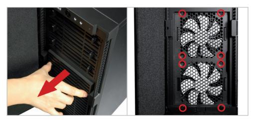
To the left and right of the fan control on the lower part of the front are two mounting holes which allow it (by using a long screwdriver) to loosen the lower screws of the 120 mm fan.
